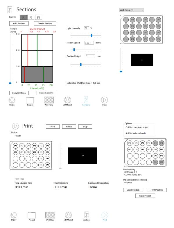
9. Once all the parameters are set, you can choose to print the complete project or only selected wells in the **Print** page. Start printing by pushing the **Print** button. The finished wells will be shown
